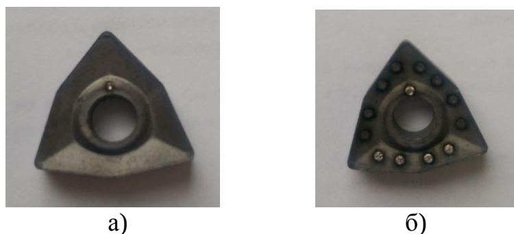
а – \tau = 10 мс, W = 8,0 Дж, \varnothing = 3,0 мм; б – \tau = 16 мс, W = 8,0 Дж, \varnothing = 3,0 мм
